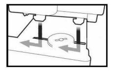
2. Attach the front of the inverter to the stand using two screws on either side.
